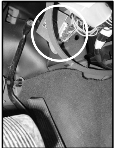
Fig. 3: '96-'01 TCU location. (Under dash)
