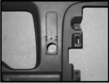
Fig. 1: Location of the mounting holes.
